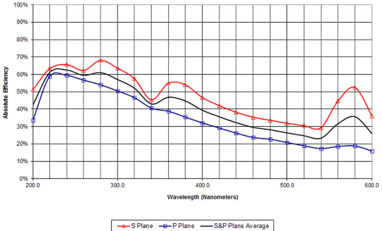
**Note:** The efficiency curve above is absolute and was measured in an in-plane near Littrow configuration (unless otherwise indicated). Efficiency curves are only representative: actual efficiency may vary significantly depending on use geometry and measurement technique. This efficiency curve is for master 5233; two masters with the same catalog number may have different efficiency curves. The uncertainty band on the data in the above efficiency curve(s) is +/- three percentage points.
